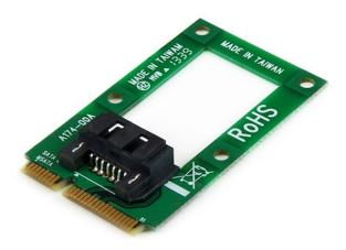
The MSAT2SAT3 mSATA to SATA adapter enables you to connect a standard SATA drive to an available mSATA port.
